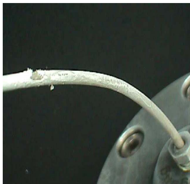
Fig. 3. Puncture of PEEK capillary, crystallization of compound on surface.
